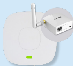
Wi-Fi access points (AP) with built in Bluetooth (BLE)
